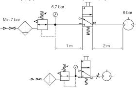
Shut-off, filtering, pressure regulation and control valve
