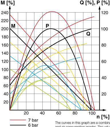
P = power M = torque Q = air consumption n = speed
